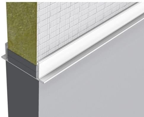
In this situation, the side of the bandraster is exposed to the heat of the fire, which is what happens in practice when the ceiling falls away. The thermal load of the construction is thus greater than when during the test parts of the bandraster are screened off, e.g. by protruding panels above the bandraster from the wall underneath. See Figure 3.2.
